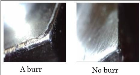
Fig2. Condition of burr of hexagon
